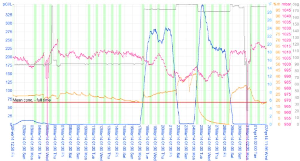
The plot shows the time interval from 2014-Feb-28 Fri 12:56 to 2014-Apr-02 Wed 11:56 (790 hours). Average radon concentration in this period is **65.8 pCi/L** ( $\pm 6\%$ ). If one includes only Mon-Fri, 07:00-15:00 (a total of 183 hours), one finds an average radon concentration of **94.7 pCi/L** ( $\pm 6\%$ ).
