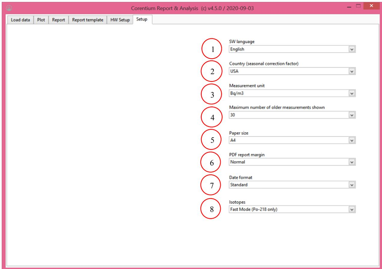
Figure 4-44 : Setup TAB - CRA SW settings
