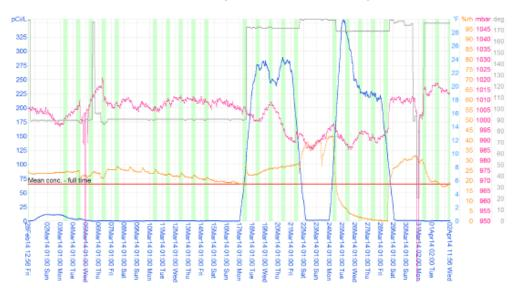
The plot shows the time interval from 2014-Feb-28 Fri 12:56 to 2014-Apr-02 Wed 11:56 (790 hours). Average radon concentration in this period is 65.8 pCi/L (±6%). If one includes only Mon-Fri, 07:00-15:00 (a total of 183 hours), one finds an average radon concentration of 94.7 pCi/L (±6%).
