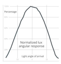
Absolute accuracy in most sensitive direction: ±5 lux ±10% within 0 - 5000 lux.
