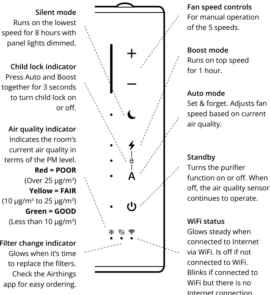
Here are the additional operations you can perform using the onboard control panel:
